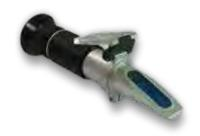
Brix is checked using a refractometer & should be performed before priming & any time syrups have been changed
