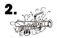
Remove spring and cup holder., Wash all parts with warm soapy water to remove dirt and wax build up. Do not bend the adjustment clips by hand.
