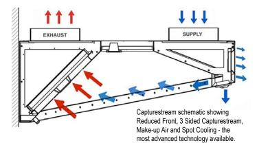
Superstream Filters more efficient at grease capture than competitive brands and with lower air rates
