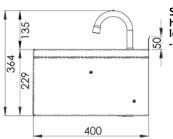
Suggested mounting height from floor level for standard use - 850mm-900mm
