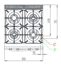
G gas connection | E electric connection | CW cold water connection | HW hot water connection | SW soft cold water connection | D drain
