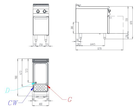
G gas connection | E electric connection | CW cold water connection | HW hot water connection | SW soft cold water connection | D drain
