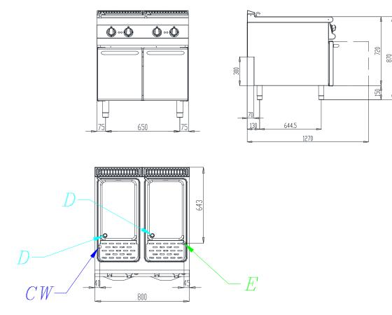
G gas connection | E electric connection | CW cold water connection | HW hot water connection | SW soft cold water connection | D drain
