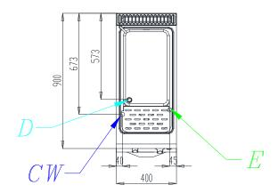
G gas connection | E electric connection | CW cold water connection | HW hot water connection | SW soft cold water connection | D drain
