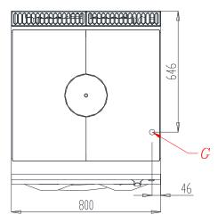
G gas connection | E electric connection | CW cold water connection | HW hot water connection | SW soft cold water connection | D drain
