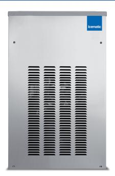
Nugget ice is generated through a vertical cylinder, with an internal turning auger which scrapes the ice from the internal surface of the evaporator, lifting it up an ice extruder which compresses the ice shavings into a cylinder.
